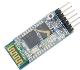
Figure 4. HC-05 Bluetooth module
